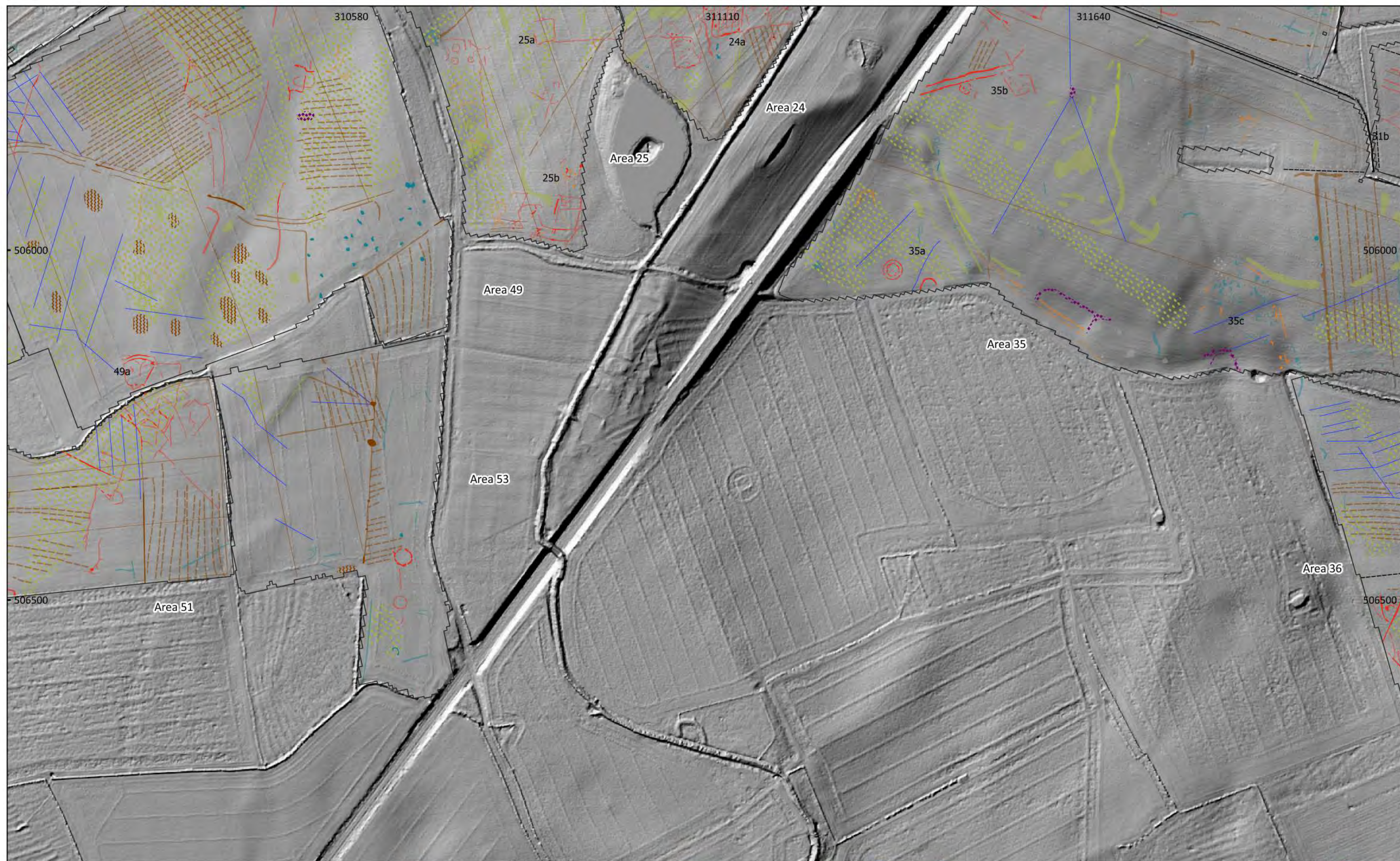
MSTF1136: Mallard Pass, DCO, Essendine, Rutland Figure 20 - Magnetic Interpretation Over LiDAR (Composite 1m DTM data visualised as hillshade plot: azimuth 35°, altitude 3°, vertical exaggeration 45°) 1:5,000 @ A3 Copyright Magnitude Surveys Ltd 2022 Contains LiDAR data: © Environment Agency copyright and/or database right 2022
